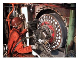
Onto a damaged area of an axle end MM-metal SS-steel, later MM-metal SS-steel 382 was applied to receive a higher surface quality. After curing, the work piece was machined down with a lathe to the desired diameter.
